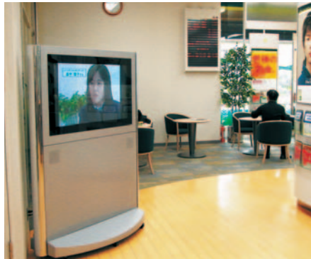
2 A plasma display (fitted in a special housing) is positioned in consideration of the movement and line of sight of customers at the entrance.
