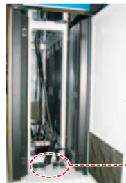
The cabinet has ample space for effective heat radiation. Several cooling fans are also installed to release heat through the slits in the side panel.
