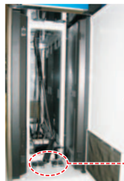
The cabinet has ample space for effective heat radiation. Several cooling fans are also installed to release heat through the slits in the side panel.
