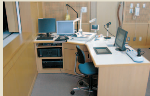
This control desk holds the control components of PCs, a calligraphic camera, and digital video cameras. The video source can be selected by touching the desired icon on the touch panel, making it easy enough for anyone to use.
